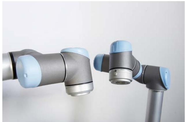
The UR 5 and UR 10 designs use KBM motors from Kollmorgen. They are integrated directly into the axis joint without a housing. Photo: Universal Robots
