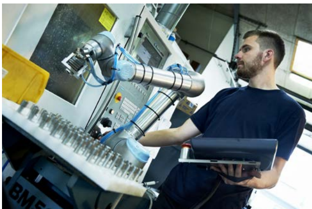
The six-axis robots are being used in processing and production facilities. The robots are easily programmed to accomplish repetitive tasks. Photo: Universal Robots
